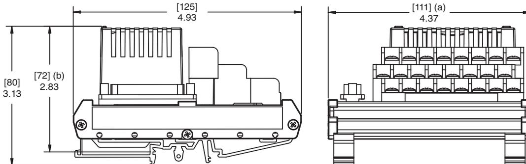
(a) Overall width – for determining DIN rail loading.
