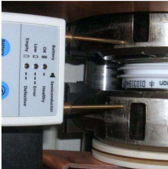
Figure 9–12 Correct measuring with FADEC 3
