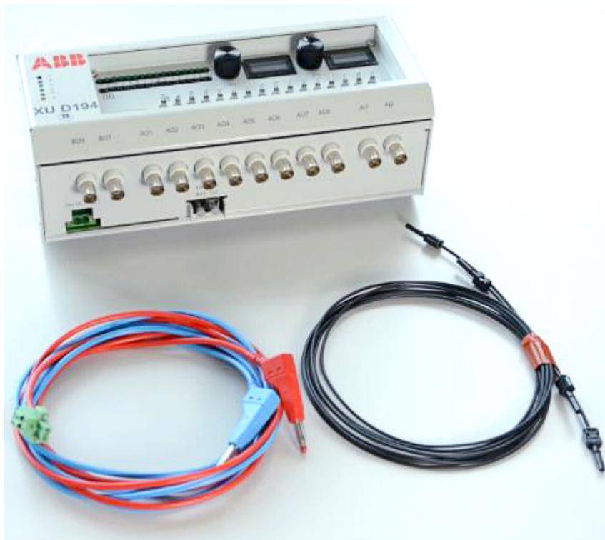
Figure 3–8 RCI-Box XU D194 with power cables and fiber optic cables
