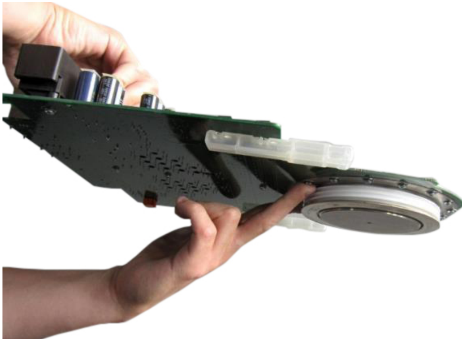
Figure 10-16 Correct handling of IGCT
