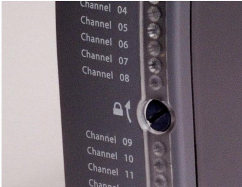
Each module carries a locking mechanism, which secures the module onto its base unit. The locking mechanism is in the form of a clamp screw, which can be seen on the front panel of the module and engaged by a quarter turn of a flat blade screwdriver. The module senses the locking mechanism position and
