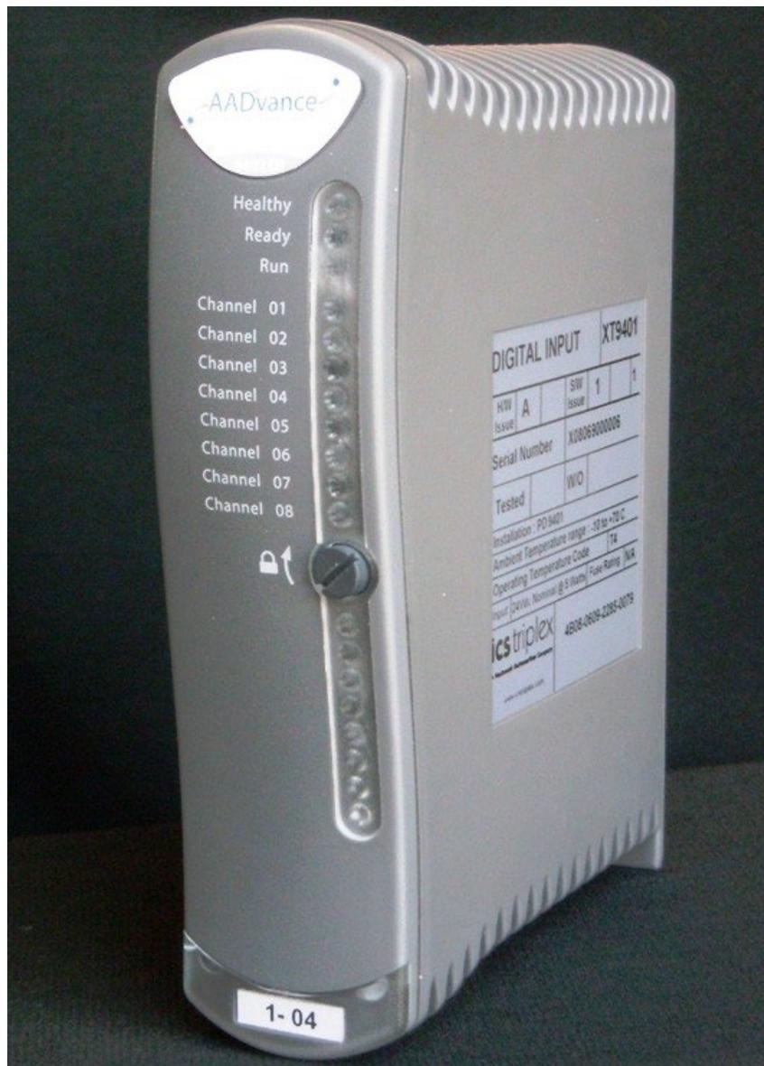
**NOTE** Standard AADvance modules have a plastic casing and are rated IP20: Protected against solid objects over 12 mm (1/2 in.) for example "fingers". There is no specific protection against liquids.
