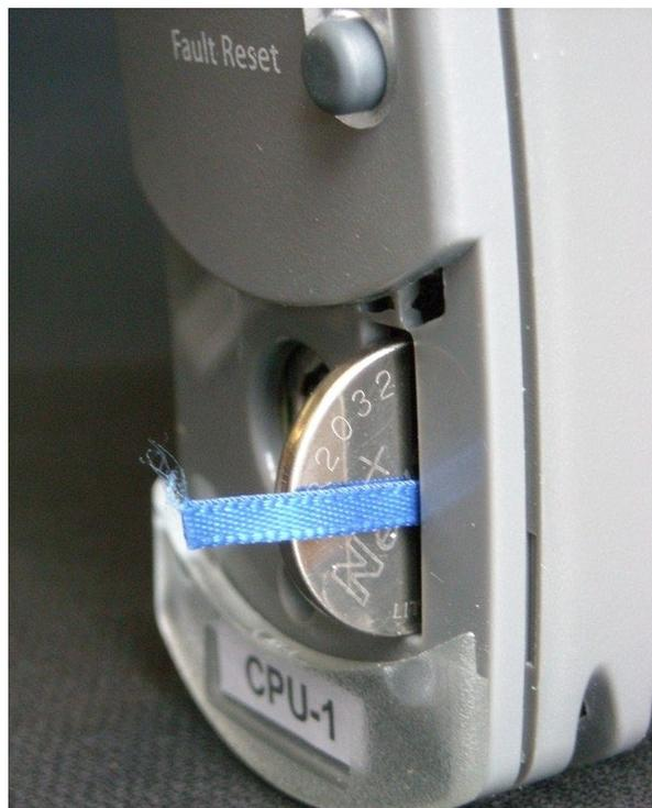
3. Insert a new battery, orientate it the positive (+) terminal to the right. Trap the ribbon behind the new battery so it can be removed in the future and then push the battery into the holder.
