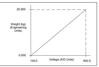
For this example, 100 to 600 is the normal resistance range, but the module will attempt to scale the inputs for a resistance that lies outside the range. If a resistance of 1000 ohms were input to the channel, the module would return a scaled channel value of 36.000. The application should use alarms or take other precautions for scaled inputs that are outside the acceptable range or invalid.
