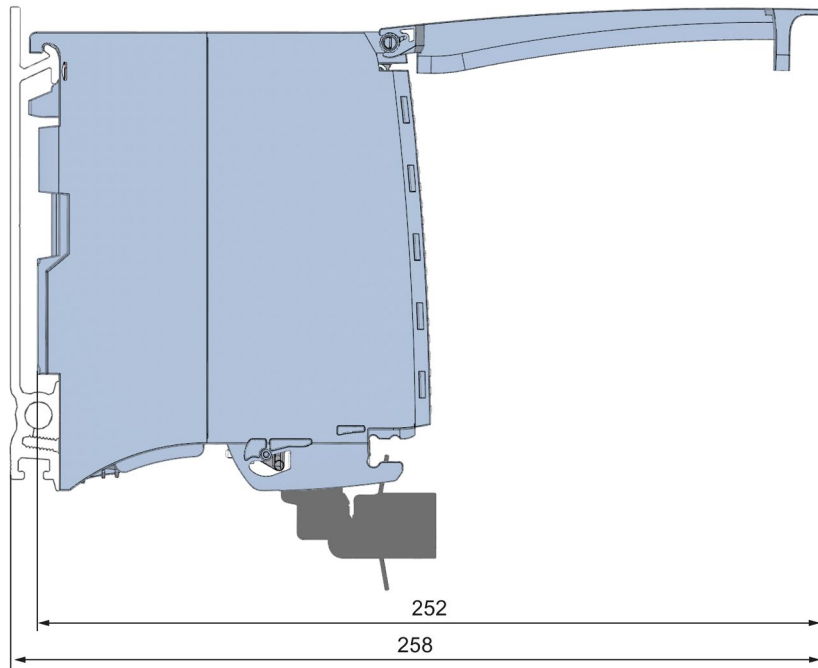
Figure A-2 Dimensional drawing of the AI 8xU/I HS module, side view with open front panel
